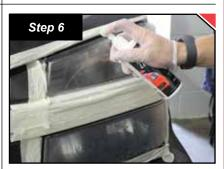
Apply and wipe headlights thoroughly with Malco<sup>®</sup> Headlight Lens Drier with clean, lint-free towel to make sure they are dry.
