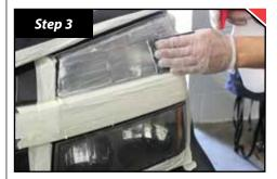
Sand the headlight lenses to a uniform appearance with P600 grit until original OEM coating is removed. During and following sanding, use water and a towel to clean the headlight and surrounding areas of all residue.
