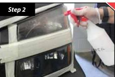
Carefully mask off area around headlights with masking tape.
