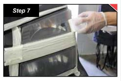
Apply Malco<sup>®</sup> Headlight Lens Sealant following the directions on the Technical Data Sheet. Allow 8 minutes for product to flatten and flash or use a heat gun on high for 1 minute.
